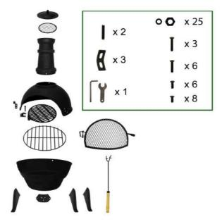
1. Screw 3x feet on with 6x large screws.
