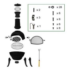
1. Screw feet on with 6x x-large screws
