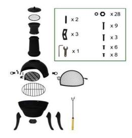
1. Attach feet with 6x x-large screws
